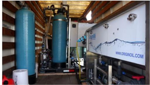
module that used electrochemical reactions for the coagulation and removal of oil, grease, and total suspended solids, which eliminated most chemical oxygen demand (COD) and biological oxygen demand (BOD), and multi-stage media filtration for polishing of the remaining fraction, including Total Dissolved Solids (TDS). The mobile treatment skid was uniquely designed to meet the discharge specifications granted by the Oklahoma City Utilities Department.
