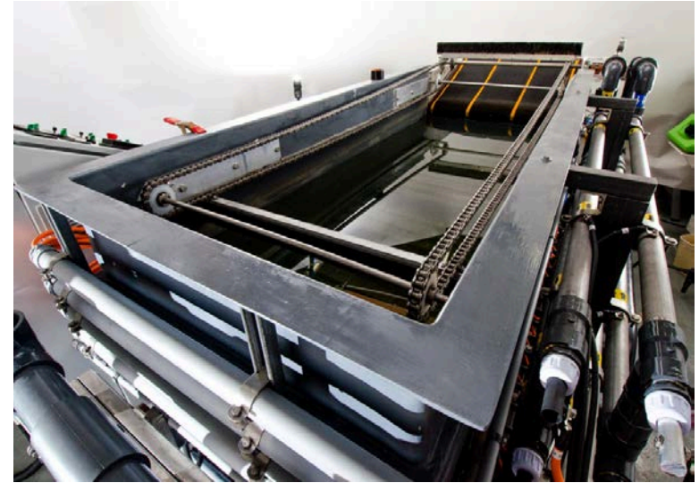
EWS PRIME P1000 With Electro-Coagulation Reactors on Right
