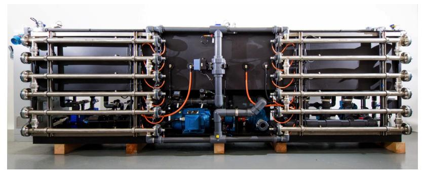
400 tons per day nominal treatment capacity – Two units fit in a 20' container
