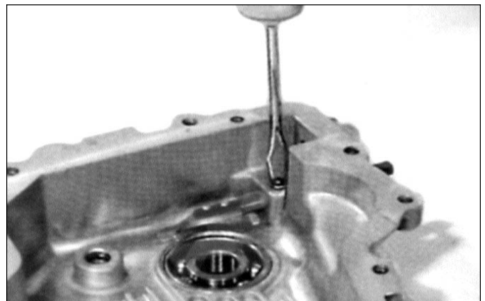
Figure 66 - Remove Governor Shaft Lock Pin
