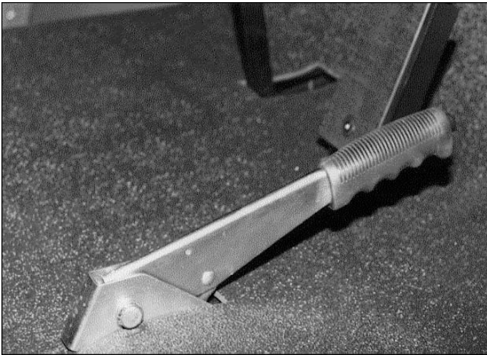
Figure 7 - Parking Brake Handle
