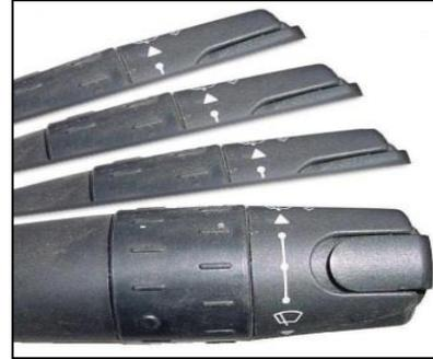
Pulling lever towards you activates the washer fluid. Pushing the switch down activates a “quick” wipe. The fluid reservoir is located under the front hood.
