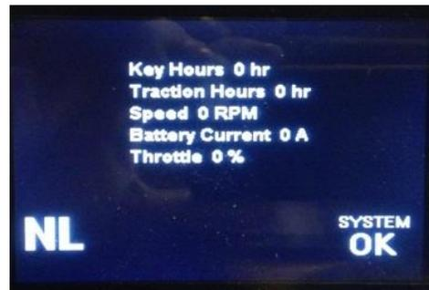
The Vehicle Status Monitor selection displays the current state of vehicle data collected at the controller
