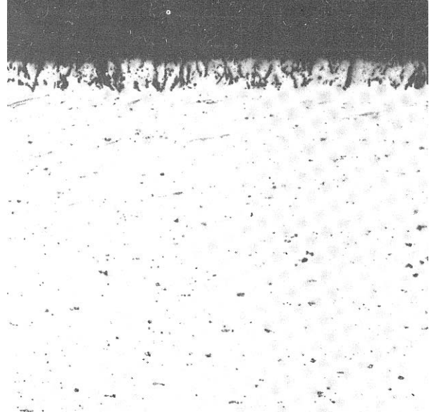
Figure 13. Oxide layer on specimen exposed to 2100°F (1150°C) for 500 hr. 75X. Unetched.
