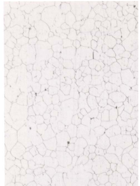
Figure 7. Microstructure (250X) of annealed INCONEL alloy 690. Etchant: 10% oxalic electrolytic.
