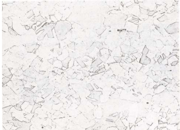
Figure 18 - Microstructure of hot-rolled, as-rolled MONEL alloy K-500. Etchant: Carapella's and glyceresia. 100X.
