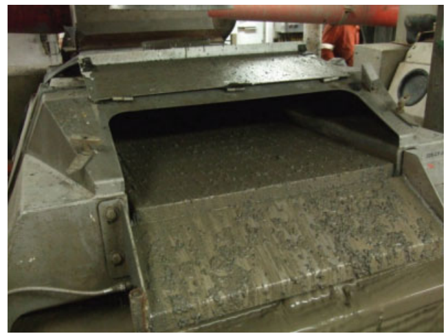
Fig. 4—Normal well returns before sand-slurry appears.
