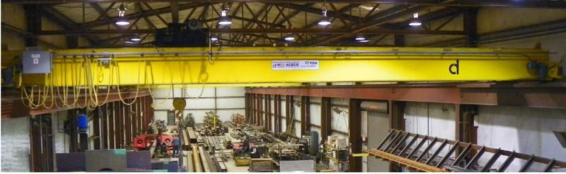
Applications for moderately rated, or Class C, cranes, include medium-grade machine shops, paper mill machine rooms, and other mid-grade manufacturing set-ups. These tools can handle five to ten lifts an hour, with an average load weighing in around 50% of their rated capacity, averaging 15 feet, not over 50% of the lift at rated capacity.
