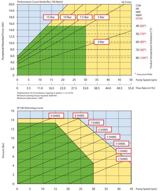
For product temperatures above 65°C and/or viscocity's above 2000 mPas use one shim less than shown
