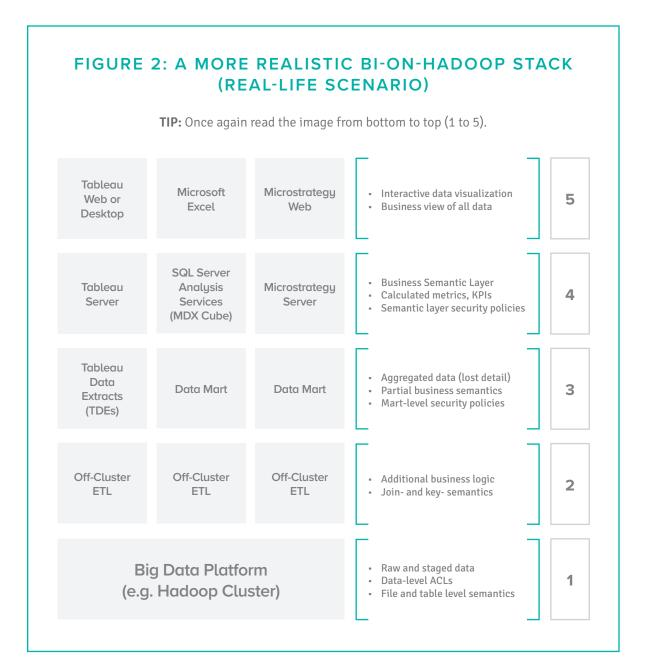
You'll notice that with the addition of multiple data consumption personae and interfaces, the cost and complexity of maintaining a functional BI-on-Hadoop operation increases exponentially. On top of the hardware, storage, and software costs discussed above, the introduction of multiple purpose-built silos creates additional challenges.
