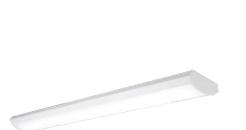
WPLD series is a versatile LED wraparound series with a streamlined, low profile design that displays uniform, soft light at up to 60% energy savings over fluorescent light sources. Mounting slots allow for installation directly into the junction box with 100° of rotational freedom. Features include suspension mount with optional mounting kit, 93 CRI, dimming to 10% and up to 115 lumens per watt.
