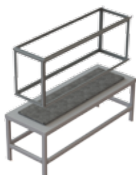
Lower frame over mounting subpanel
