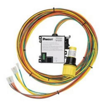
Voltage indicators are tools that can warn of hazardous voltage but cannot be used to confirm if the equipment is de-energized. The VeriSafe AVT is a permanently-mounted test device designed to verify that a circuit is de-energized prior to opening an electrical enclosure.
