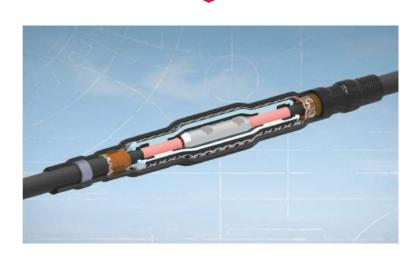
TE Connectivity's (TE) Raychem CSJA "All-In-One" joints offer a reliable, fast and easy-to-install jointing system to assure and maintain high network reliability. TE's Raychem CSJA are designed to splice tape shield, wire shield, LC shield, UniShield, JCN and flat strap shielded cables from 15 kV up to 35 kV.
