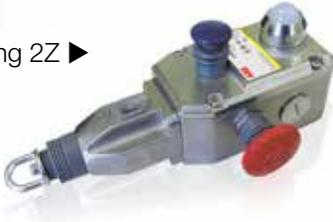
ABB JOKAB SAFETY **Line Strong** switches are designed to be mounted on machines and sections of conveyors which cannot be protected by guards. In contrast to traditional mushroom head type Emergency Stop buttons, Safety Rope Pull Switches can initiate the emergency command from any point along the installed rope length and provide robust emergency stop rope pull protection for exposed conveyors or machines.
