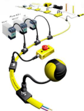
The **Pluto AS-i** system is distinguished by its special yellow profile cable. The cable connects all sensors, transducers and actuators on the network to a supervisor system. The component parts of a system can include both non-safe and safe products. This means that both operational and safety related products can be mixed in a network. The bus system drives a Supervisor-Subordinate (node) configuration where each I/O module corresponds to a common supervisor.
