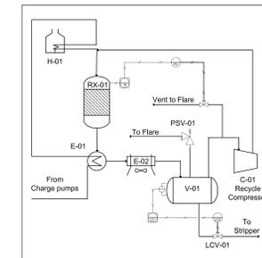
Figure 4: During an upset event due to the loss of the compressor, the relief load is not expected to be any larger as the recycle gas is lost. This source is not a feed source since it never enters or leaves the system. Also, the de-pressuring valve on the suction line to the compressor may open to vent to flare if a high temperature reading occurs.
