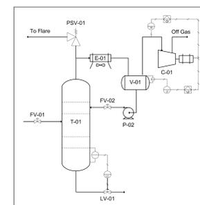
Figure 5: During a partial loss of cooling in E-01, the T1 on the suction to C-01 may trip the motor to shutdown due to a high temperature reading. Due to the loss of the compressor, the credit for partial cooling cannot be taken as the vapor would accumulate and vapor lock the overhead condenser; thus, the partial loss of cooling would result in a completely blocked overhead outlet.
