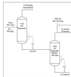
Figure 3: During the upset event, a liquid inventory needs to be analyzed. If the upstream vessel cannot overflow the downstream vessel, then gas blow-by may occur and the valve would be passing the overhead vapor downstream. Credit may be taken for the minimum vapor leaving and potentially sizing the control valve with two-phase as it is likely seeing liquid and vapor on the inlet.
