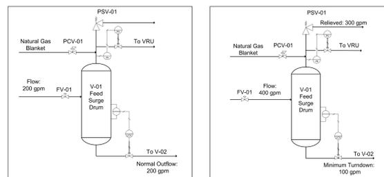
Figure 2: During normal operation (on the left), the pressure is regulated by the natural gas blanket on the overhead; thus, there is normally no vapor flow. During the upset condition (on the right), the control valve would fail open and credit can be taken for the minimum turndown rate through the bottoms control valve. Credit cannot be taken through the vapor line as there is normally no flow.
