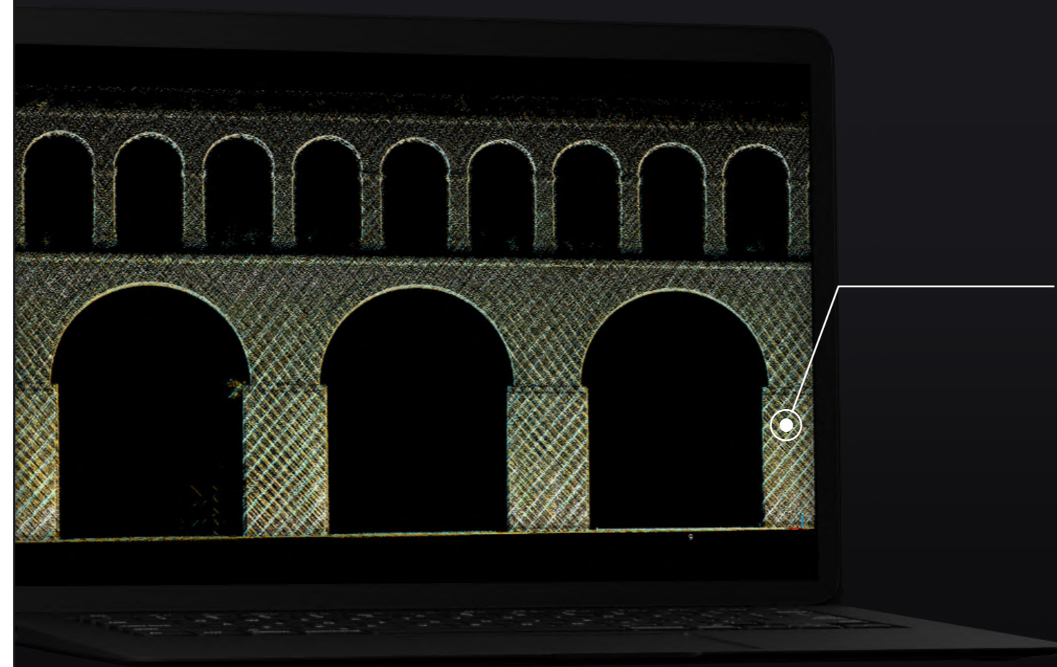
Strip Adjustment results Point cloud after precise strip adjustment process
