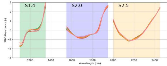
Example spectra from eight silage samples collected with three NIRONE variants. Each spectrum is a sample average over 60 scans and preprocessed with SNV.
