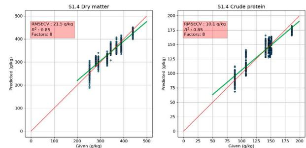
Predicted vs. reference plots for Dry matter and Crude protein determination using NIRONE S1.4
