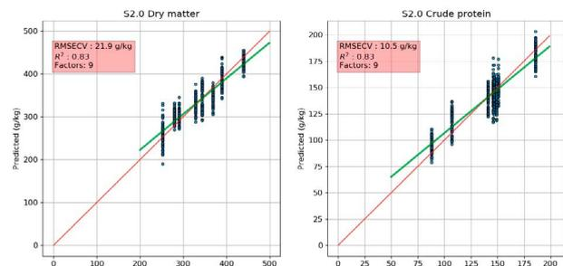
Predicted vs. reference plots for Dry matter and Crude protein determination using NIRONE S2.0
