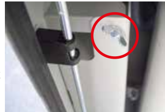
Opening the washing liquid container (wing screw)
