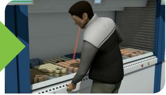
The operator returns to the waiting cart, just a few steps away. Orders are associated with a specific tote on the cart, each of which is also equipped with put-to-light modules that illuminate with the put location and required item quantity.
