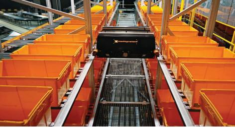
Many goods-to-person systems combine multiple technologies to optimize flow, for example, using AS/RS to store overstock. Instead of delivering to the end of the aisle, the AS/RS automatically replenishes adjacent carton flow rack holding the fastest moving, manual-pick items, and goods-to-person shuttle systems that hold three days of inventory.
