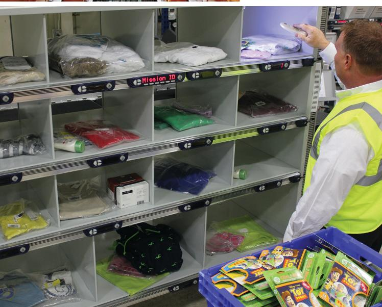
At the person end of a goods-to-person system, order put walls (shelves of cubbies that separate individual orders) can be equipped with light-directed pick or put modules to indicate which SKU goes to which order and in what quantity—maximizing throughput and improving accuracy.
