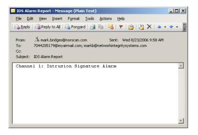
It can be seen that the email alarm has more information (system ID, channel parameters, action taken by Interceptor) than the SMS alarm. However, some devices such as SMS cell phones and pagers may not be able to correctly display the email message as the message would have too many characters. The SMS target is provided for such devices. We have found that the SMS target is the best one for use with an alphanumeric pager.
