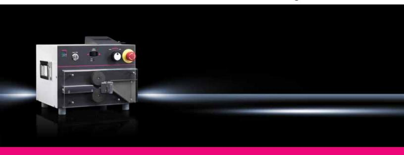
Semi-automated machine for cutting wires to an individually adjustable length.
