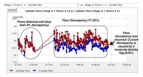
• Compressor flow increased by 4.56 MMscfd after the pocket repairs. The fixed volume pockets were actually able to close all the way without any leakage.
