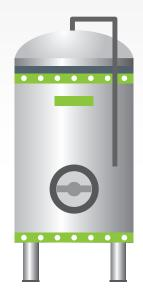
Bright tanks are where clarified beer is stored after it has been filtered and before it gets bottled or placed in a keg / cask. It is not uncommon for a quantity of beer from one production batch to remain in a bright tank when a new production batch is added to the tank. As a result, two separate batches of beer that would ordinarily be tracked with two distinct lot numbers, have now effectively become blended into a single "combined" batch, which is then packaged and sold to customers.
