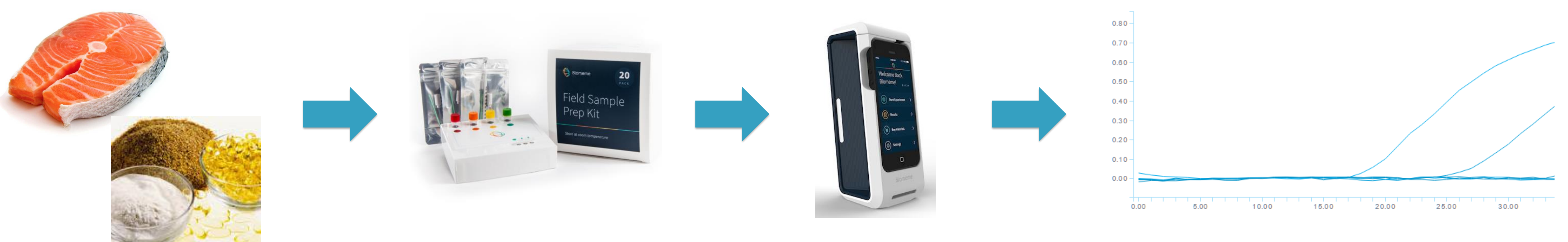
Figure 1. Steps for simplified DNA authenticity. Samples are taken from seafood or NHP using sterile, disposable tweezers or swab, subjected to a 5-10 minute DNA extraction protocol and added to the corresponding species-specific real-time PCR assay. Lyophilized reagents and a hand-held instrument allow field-testing in less than 90 minutes. Results are displayed on the instrument showing presence or absence of the target species, and are automatically uploaded to a secure web portal for additional analysis.
