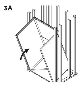
Return the fixture to the upright position, carefully ensuring that the drain fits properly in the boxed out area.
