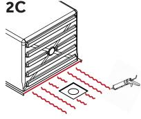
Option B: Apply construction adhesive along the front threshold and onto the floor perpendicular to the support plate rungs. There should be approximately 3" of space between lines of adhesive.
