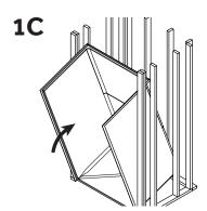
Place the fixture in the framed alcove and ensure that the floor is level and that the walls are plumb. The floor must be leveled prior to installation if it is greater than 1/8" from level.
