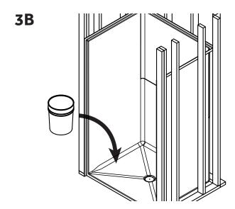
Evenly distribute weights on the fixture floor for the amount of time recomended by the adhesive manufacturer. At least 120 lbs should be used for this step. This is approximately the weight of three 5-gallon buckets filled with water.
