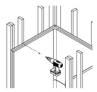
To secure the fixture to the stud walls, pre-drill holes every 16" along the vertical flanges and one hole per stud along the horizontal flanges. Nail or screw the fixture to the wall at each hole.
