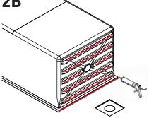
Option A: Apply construction adhesive along the front threshold and along each rung of the support plate.
