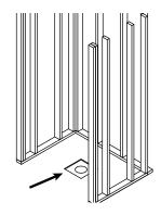
Drill a 6" diameter drain core through the subfloor centered with the fixture drain as shown in the product specification sheet. Box out a 1/2" deep, 10" x 10" square centered with the drain core.
