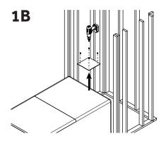
Remove the 12" x 12" board used to protect the drain during storage from the back of the fixture.
