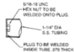
Detail of Internal Nut
