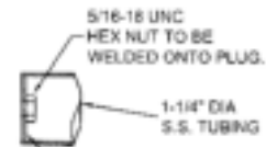
Detail of Internal Nut
