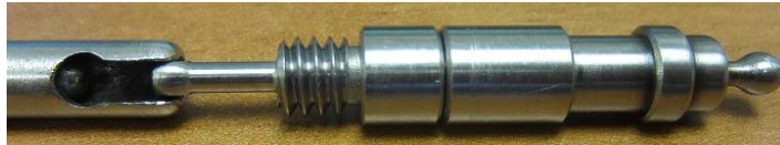
FIGURE 11 – JUMPER IN RETRIEVAL MODE INSERTING INTO TIF CONNECTOR. ROTATE JUMPER 90° AND SLOWLY PULL TO RETRIEVE
