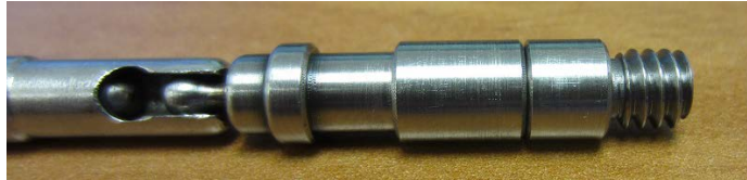
FIGURE 8 – SHORT LENGTH JUMPER CONNECTED TO TIF SOURCE CHAIN
