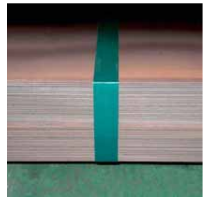
Strapping of steel plates
