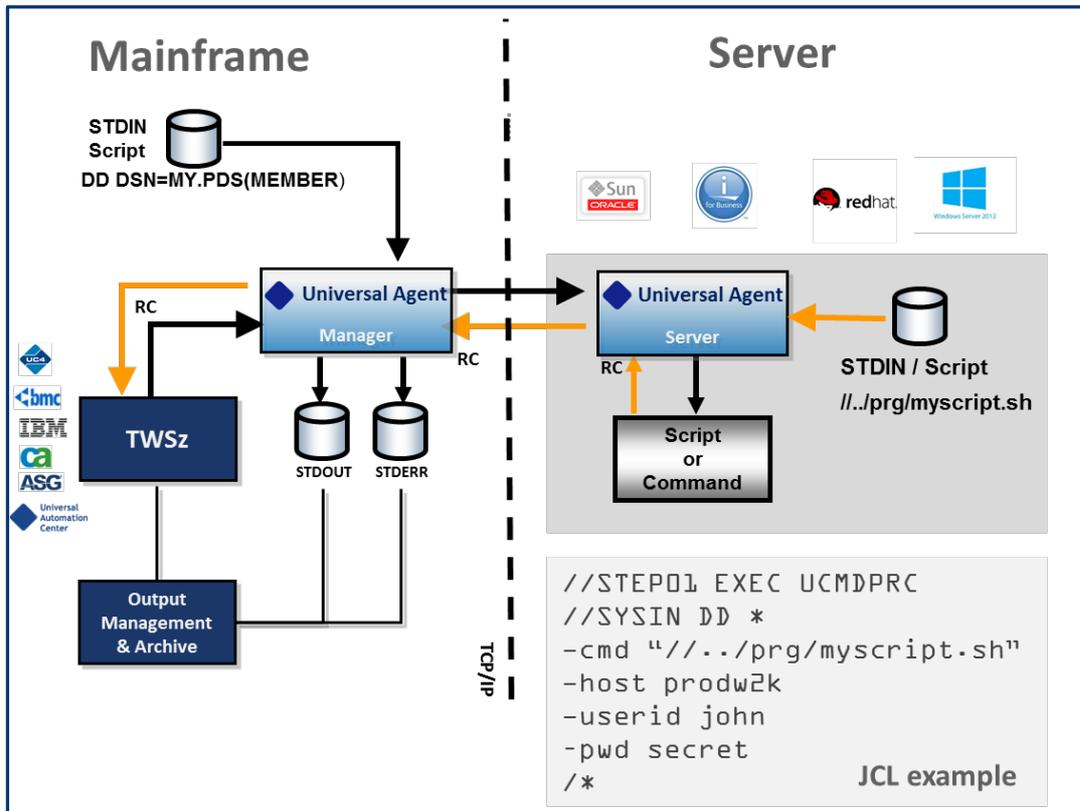
Figure 3: Triggering a UNIX script from the mainframe via Universal Agent
