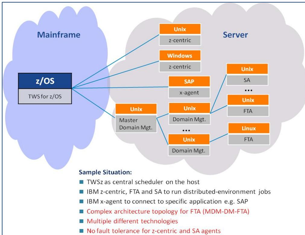
Figure 4: TWS/z workload controlled by different types of agents
