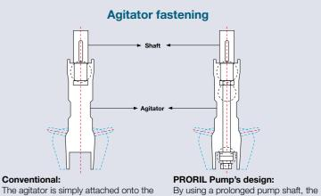
end of the pump shaft. As the agitator is agitator is fastened at three separate points, ensuring that the agitator cannot loosen itself or come off during use.
