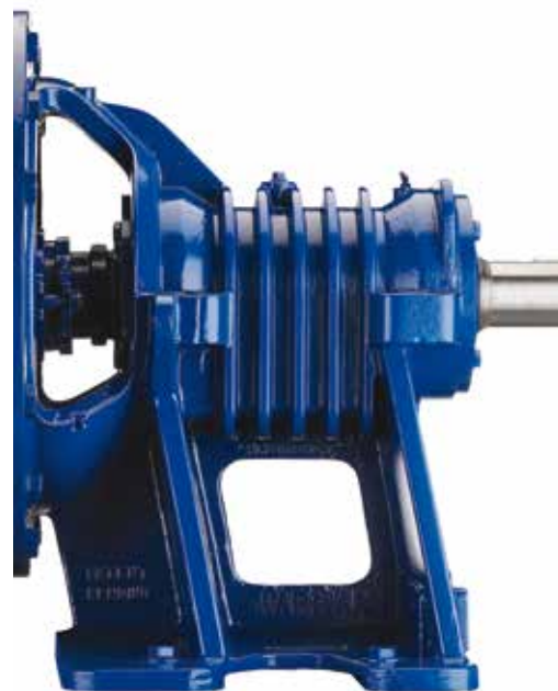
New one-piece WBH® bearing frame design for correct alignment of bearings, seal and impeller to front liner. Less part count. More robust.
