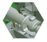
Bi-directional, loaded single mechanical seal with elastomer bellows, with or without knife edges. Seal rings of SIC. Elastomer material also FDA-approved upon request.
