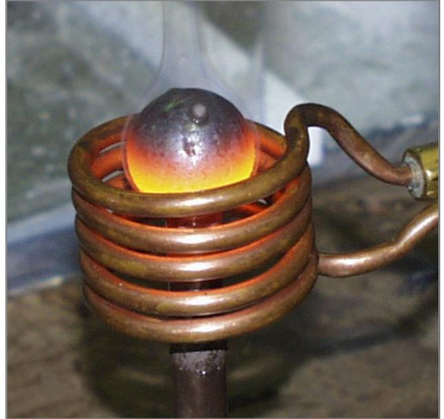
Steel to steel brazing of part of a regulator used in the oil industry. 200 kHz at 8 kW for 9 seconds to 732°C (1350°F).
