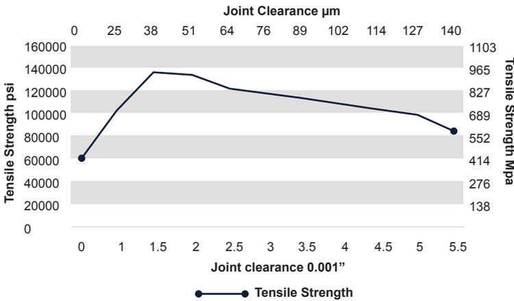
The optimum braze joint strength occurs with a part joint clearance between 25µm (0.001") and 125µm (0.005"). Data from Lucas Milhaupt.
