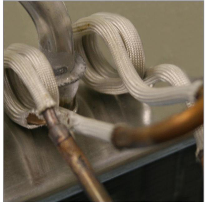
*Replacing torch brazing of aluminum tubing to air conditioning evaporator. Using flux cored aluminum braze rings and a split helix induction coil for easy access to the joint area. 5 kW at 260 kHz for 12 seconds to 565°C (1050°F).*
