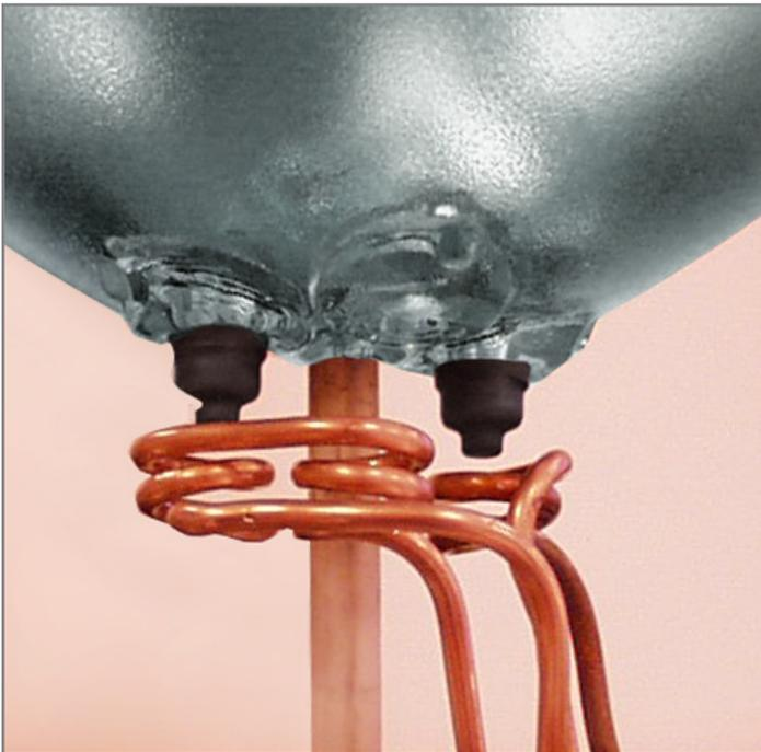
*Replacing torch brazing with a multi-position helical coil to induction braze two or three nickel plated steel ferrules to nickel plated pins from an Automobile light bulb. 8 kW at 360 kHz for 6 seconds to 620°C (1150°F).*
