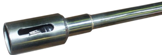
*Sensor assembly using a 3/8" diameter stainless steel tube brazed to the 1/2" diameter stainless steel sensor body. 3.5 kW at 300 kHz for 20 seconds to 732°C (1350°).*
