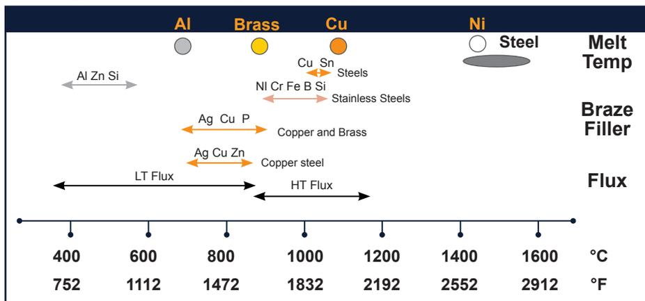
Filler and flux operating temperature ranges for typical materials used in brazing steel, copper, brass and aluminum.
