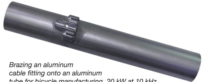
*Brazing an aluminum cable fitting onto an aluminum tube for bicycle manufacturing. 20 kW at 10 kHz for 45 seconds to 482°C (900°F) using stick fed braze. Two parts were brazed simultaneously in a two position coil.*
