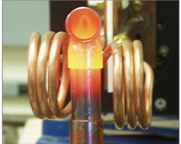
*Replacing torch brazing on a copper elbow to copper pipe using a split helix coil. 7 kW at 190 kHz for 90 seconds to 760°C (1400°F).*
