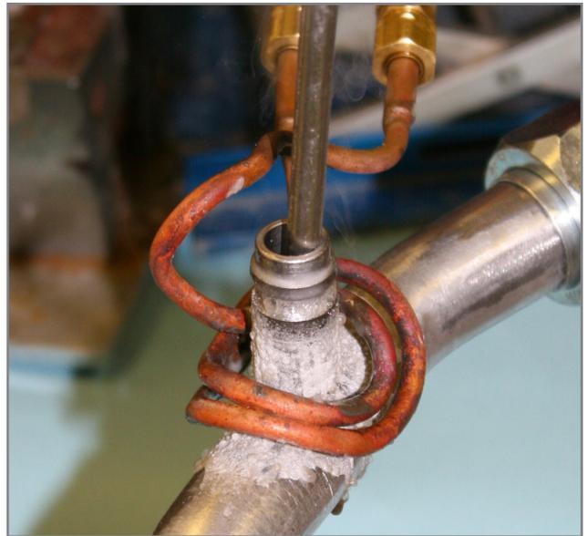
Brazing steel tube fittings used on trucks. 300 kHz at 3 kW for 45 seconds to 732°C (1350°F).
