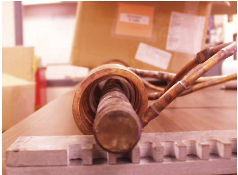
End view of stainless steel pipe passing through coil
