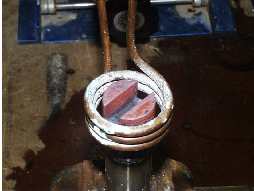
Motor shaft in coil starting to heat
