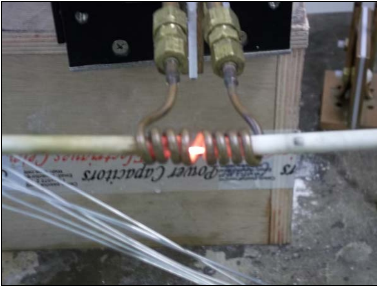
The wire being heated inside the induction heating coil
