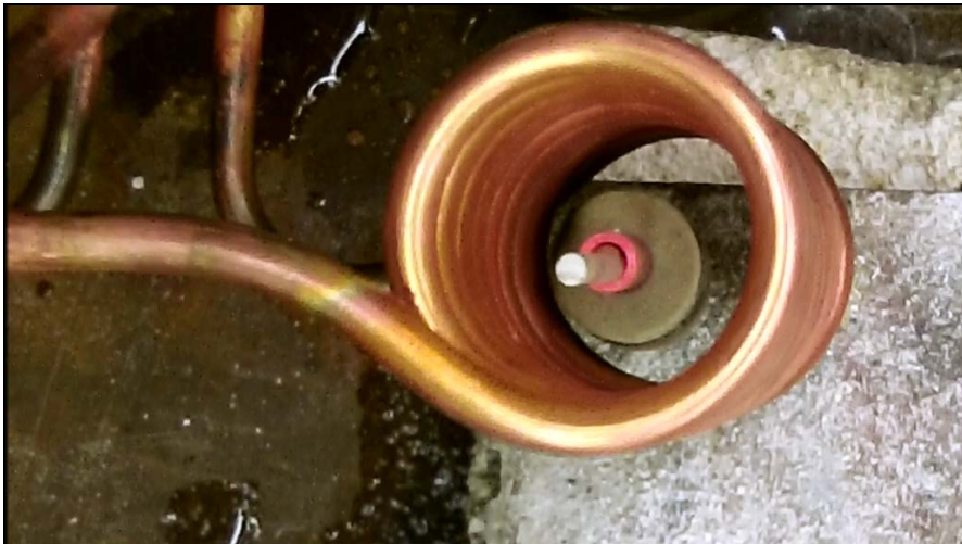
The smallest copper tube during heating.
