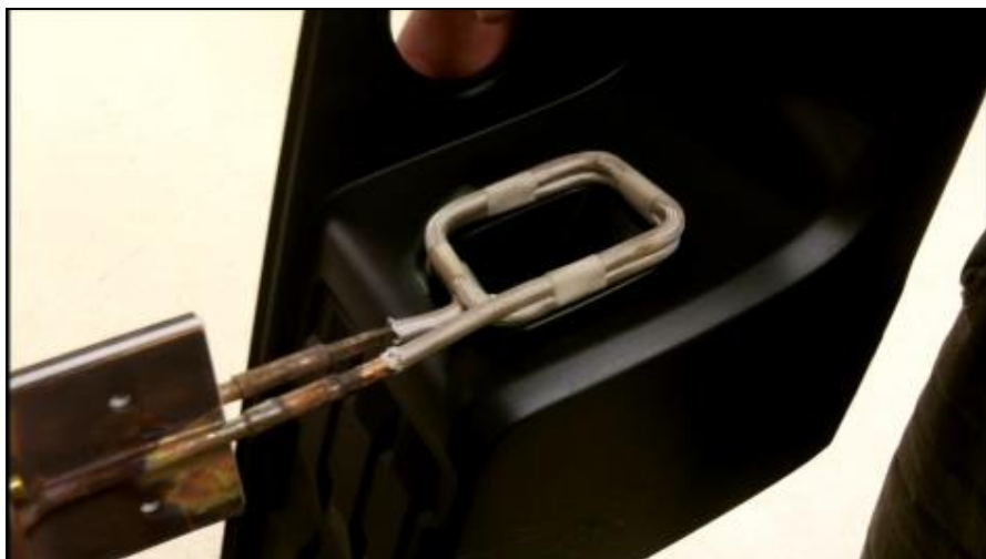
The coil design used to generate the magnetic field.
