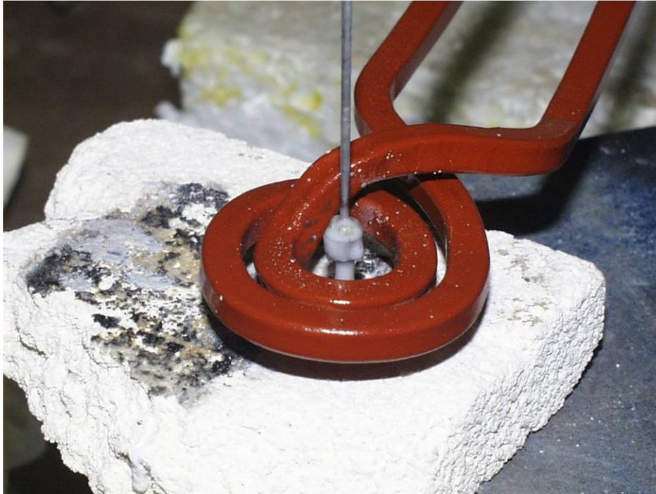
One end of assembly in coil for brazing
