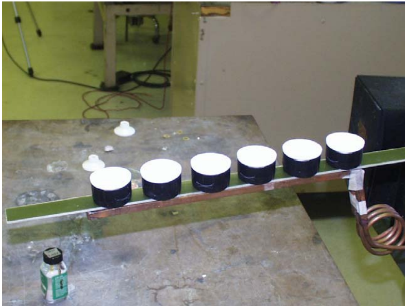
The 12" coil with six caps (top and bottom) and six aluminum disks (not seen in picture) prior to heating
