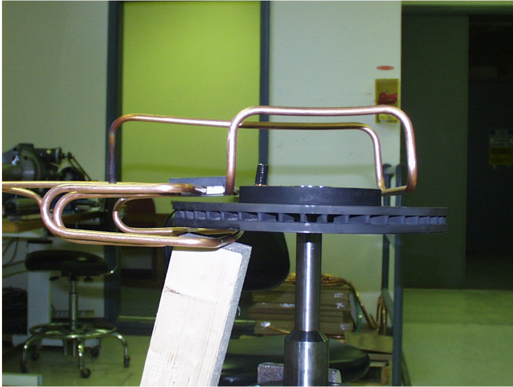
Coil designed to promote uniform heating
