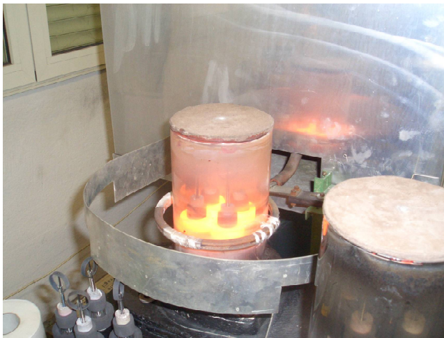
Susceptors being heated in Nitrogen atmosphere
