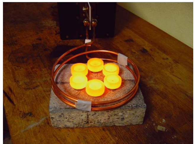
Placement of susceptors showing uniform heat pattern
