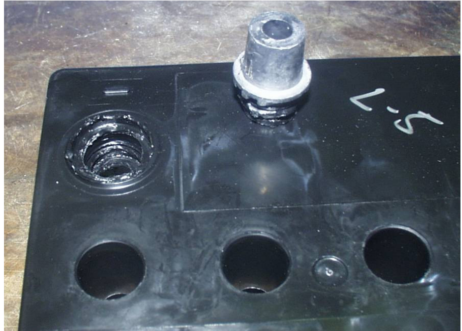
Terminal after it has been heated and removed
