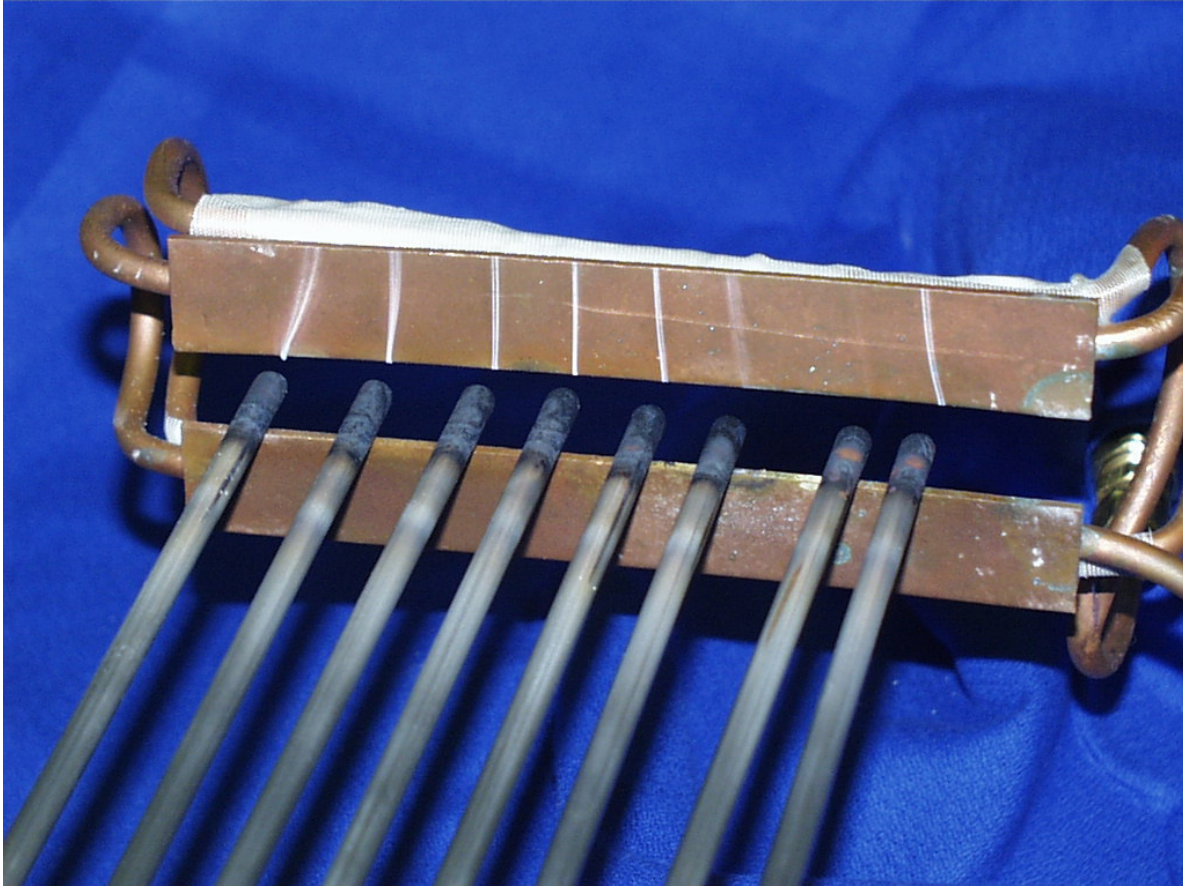
Multiple wires heating in coil for hot heading
