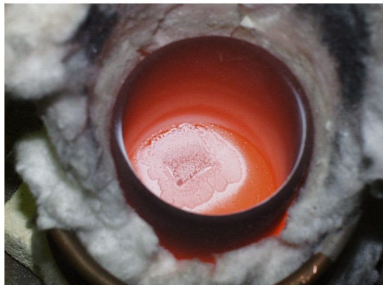
Crucible showing melted silicon
